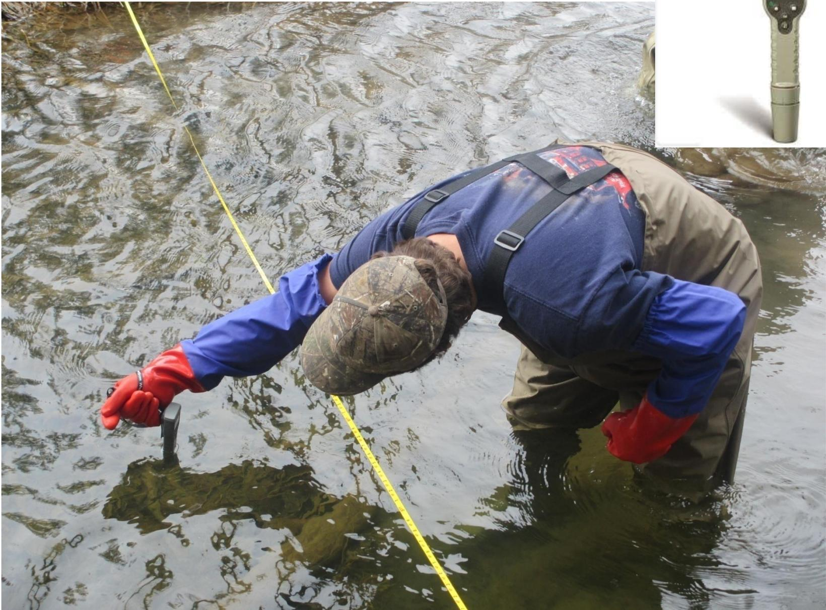
**pH was measured using a YSI pH10 Meter**
