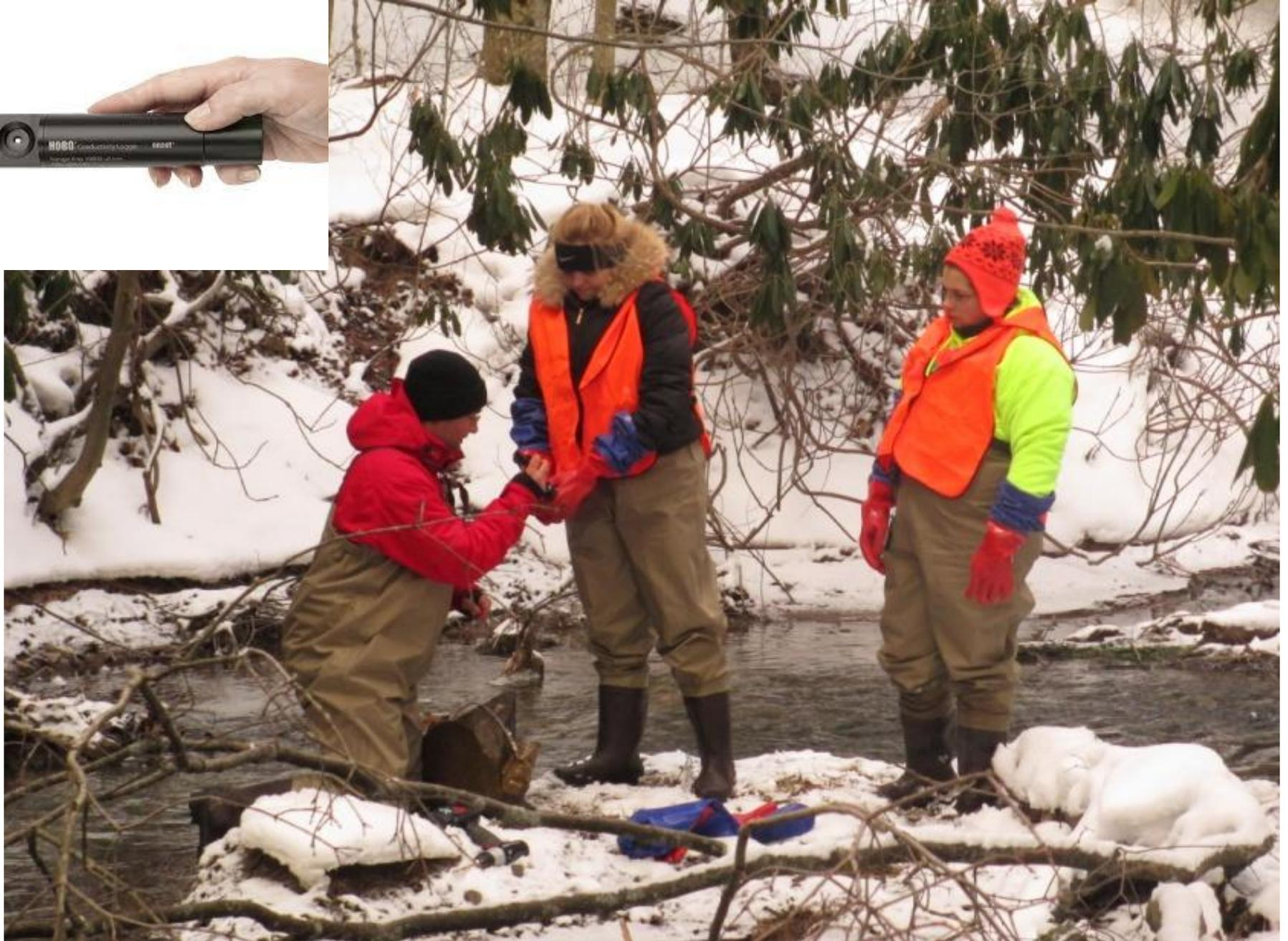
**Rock with HOBO monitor is pulled from stream**
