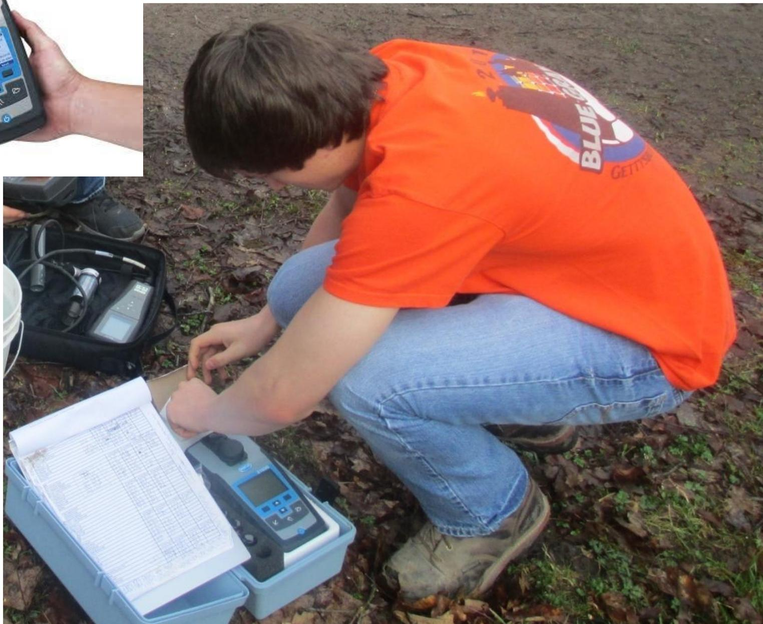
**Turbidity being measured using a Hach Turbidimeter**
