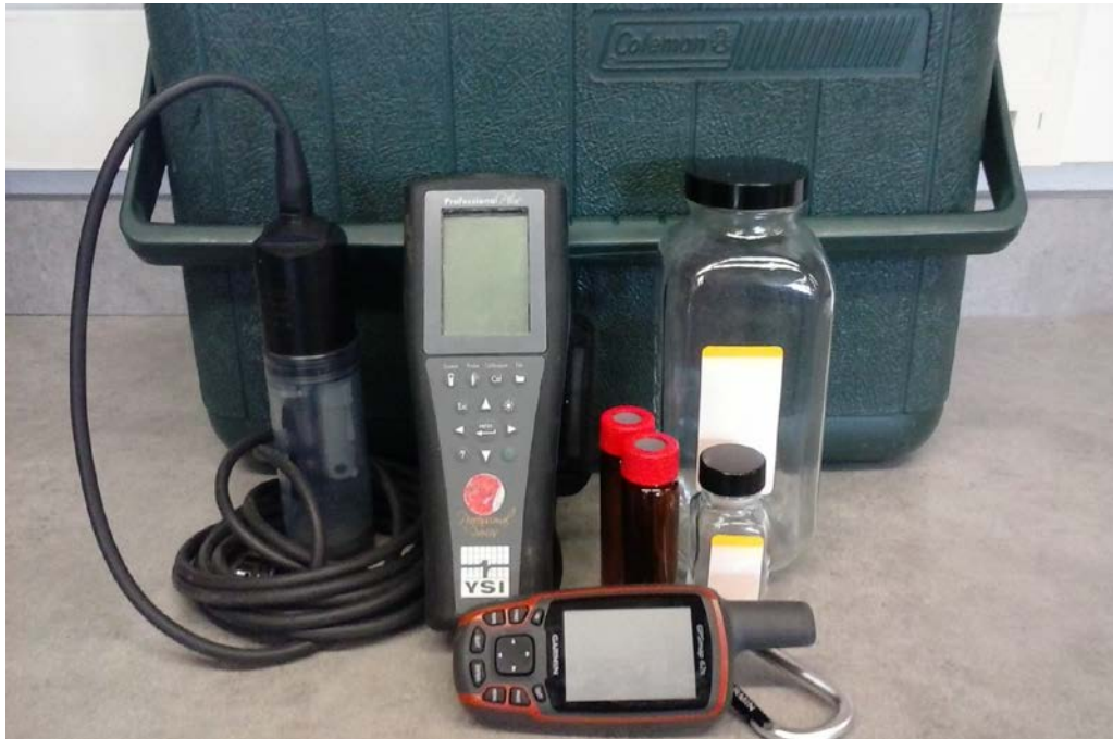
The Set Up For Field Analysis: YSI, GPS, Cooler, Vials
