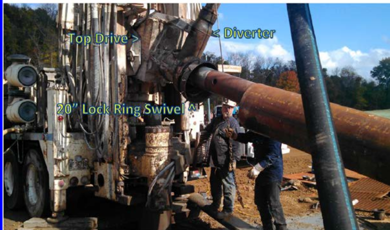
Concentric Casing Drilling Rig: inner drill pipe rotates an air percussion hammer/bit inside 94# 20" which is locked in place with a lock ring swivel and rotated independently of the inner drill pipe
